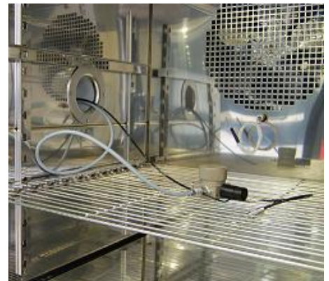
Interior of FitoCal with external humidity calibration equipment
